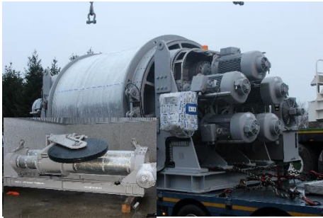
RA winch with AHC and speed of 3m/s
