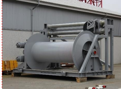
12.000m traction winch, with AHC and speed of 3m/s
